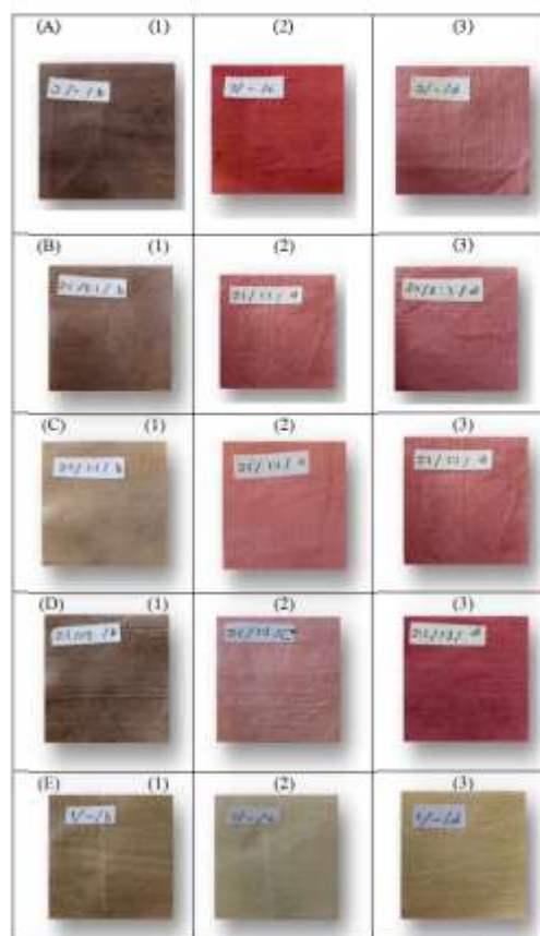
Fig. 6 Physical Appearance of: (a) A; (b) AC1; (c) AC2; (d) AC3; (e) C Dyes with Fixer: (1) iron (II) sulfate, (2) alum, and (3) calcium oxide
